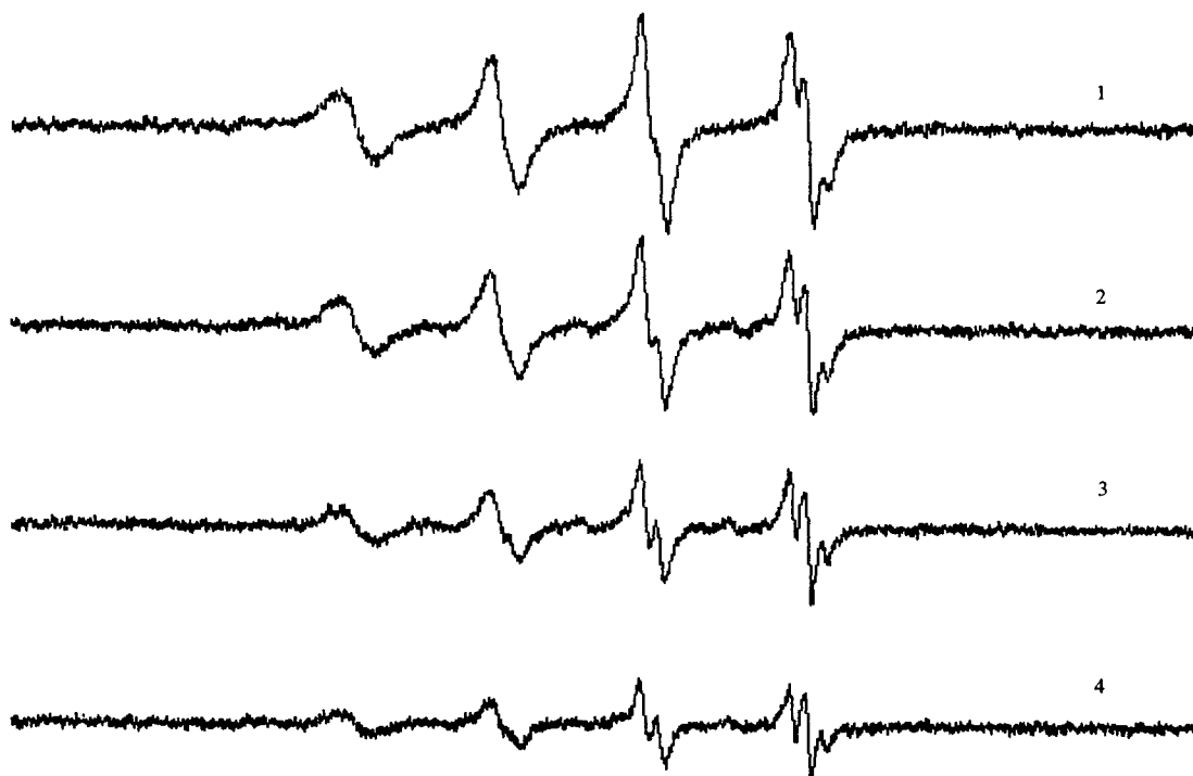
Fig. 4. Changes in the EPR spectrum of an aerated toluene solution of \text{Cu(dtc)(dtp)} complex ( 1 \times 10^{-3} \text{ mol dm}^{-3} ) following visible light irradiation. Spectra before (1) and after 0.3 min (2); 1 min (3) and 2 min (4) of irradiation.
